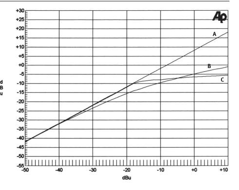
Diagram 2 shows various cut and boost settings of the air band filter.
