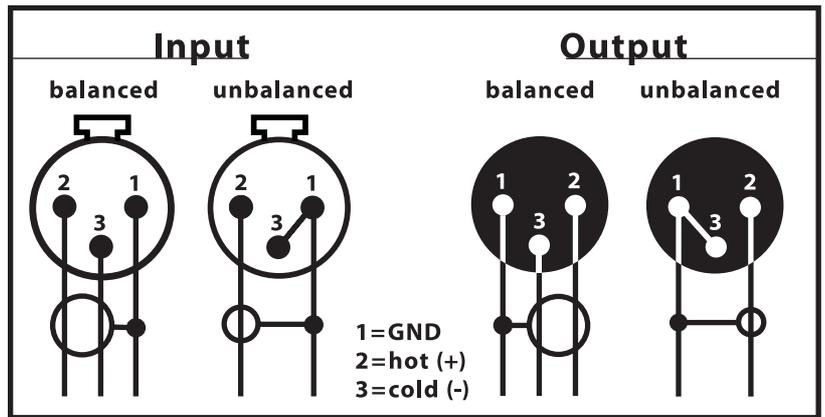
Both output stages operate in parallel, so it is possible to connect two different destination units simultaneously, for example to record to two different media at the same time or split the output between a mixer and effects processor. However, only one type of input (jack or XLR) should be connected at a time – the Tube Vitalizer is not intended to be used as a mixer!
