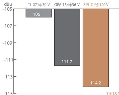
When it comes to volume, the 120-volt technology exhibits a performance that is twice that of common components and circuits, in regard to maximum level and dynamic range, with values that are approximately 10 dB higher. THD measurements of the SPL op-amps show a difference of more than 3 dB compared to the OPA134 at 36 V — in terms of sound pressure level, that corresponds to an improvement of more than 50%.
