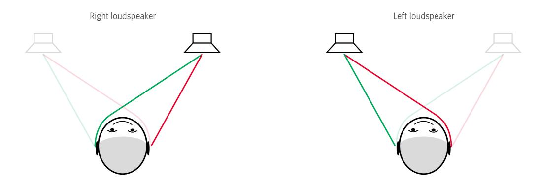
It arrives later because the signal travels a distance of approx. 340 meters per second and the distance from the right speaker to the left ear is longer than it is to the right ear. It is quieter and does not deliver the full frequency range, because the signal of the right speaker does not directly arrive at the left ear but is partially reflected and absorbed by the head.
